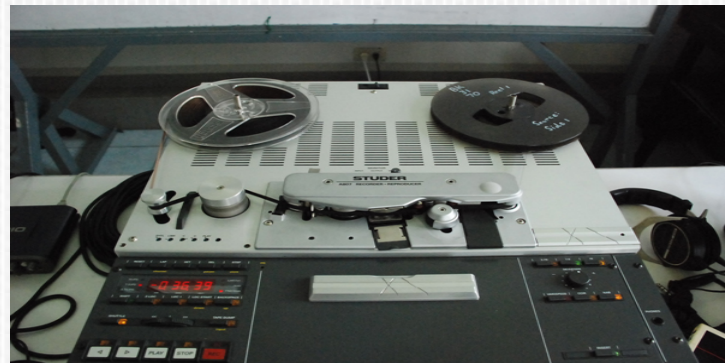
left: preparation of space for Audio Conservation Laboratory; right: Digitization Equipment (Struder A807)
